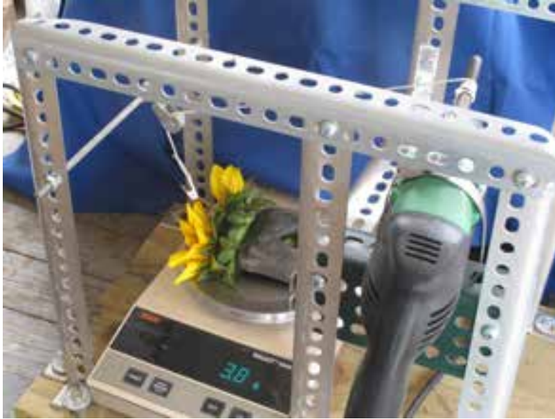
Fig. 5. Petal pulling apparatus, showing an electric drill, to which a pulley mechanism is attached, so that the direction of pull is in the direction of attachment of the petal. The flower head is resting on the scale, held down by a lead weight.
