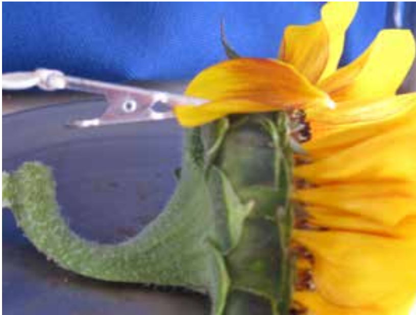
Fig. 6. Halved sunflower head with petal clamp pulling the petal backwards. Note that the green sepals of the head have been removed with scissors to allow the petal to be pulled at an acute angle without impedance.
