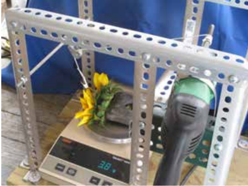
Fig. 6. Petal pull apparatus showing a sunflower head lying on a balance pan, with petal attached to a clip, being pulled upward by the string attached to the shaft of an electric drill.
