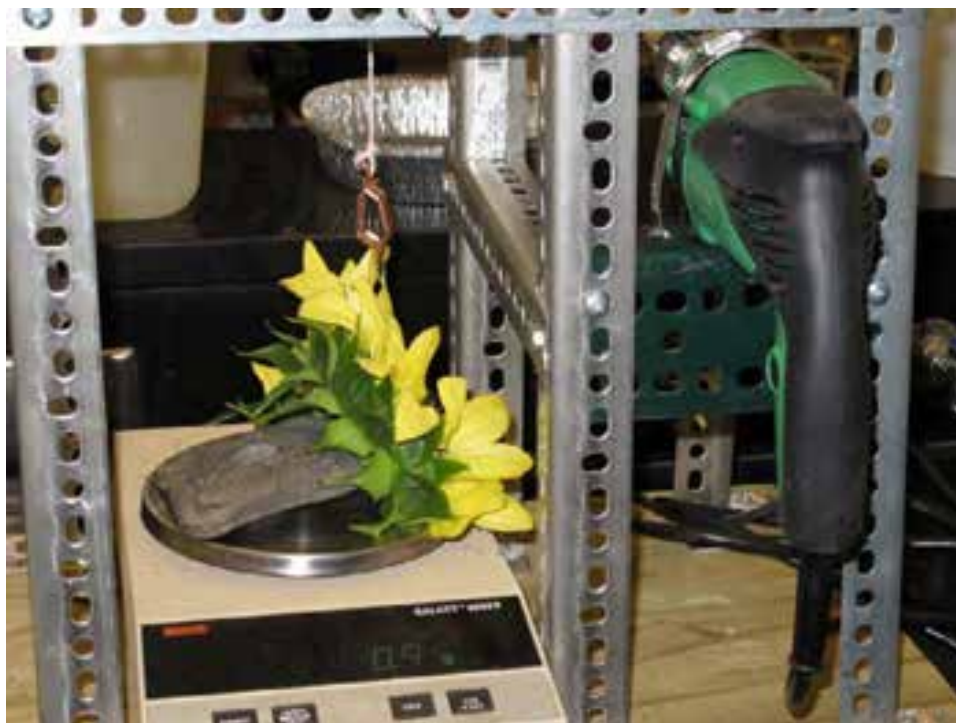
Fig. 10. Petal retention force measuring apparatus, consisting of a balance(left) on which a sunflower head is placed, held down by a weight. A clip attached to a petal is pulled upward by a string attached to an electric drill (right). The force needed to detach the petal is indicated by a decrease in weight on the balance.
