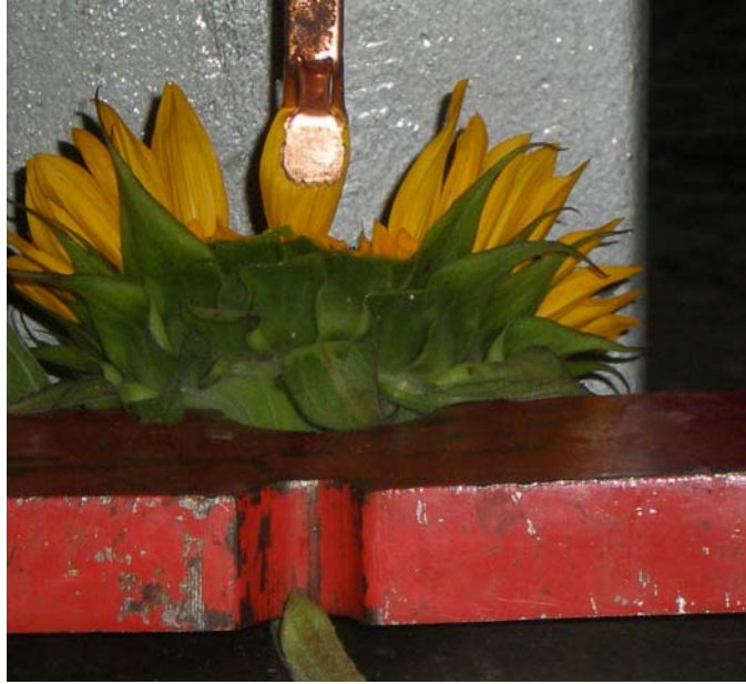
Fig. 8. Petal break strength meter used to measure the force necessary to pull an individual petal out of the sunflower. The flower is resting on a scale, connected to a computer which measures the force reduction on the load cell as the petal is pulled slowly upward.
