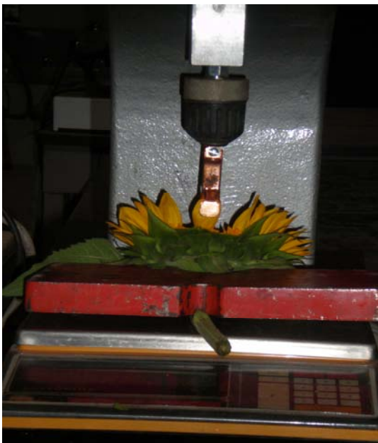
Fig. 9. Overall image of the scale, sunflower stem and flower, petal holding clip and arm attached to the arbor press.
