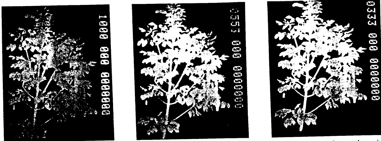
Fig. 2. A series of the scanned image of an ash tree as the appropriate threshold level is achieved. (Left) 100.0% white (percent shown at the top right side of each frame). (Middle) As the threshold is decreased, less of the background image reads as white. (Right) Just the actual tree canopy is illuminated by scan lines (representing 33.3% of the entire frame).
