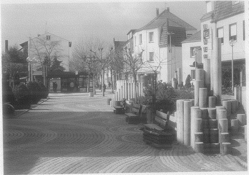
A German woonerf features concrete rounds laid on gravel to facilitate percolation.
