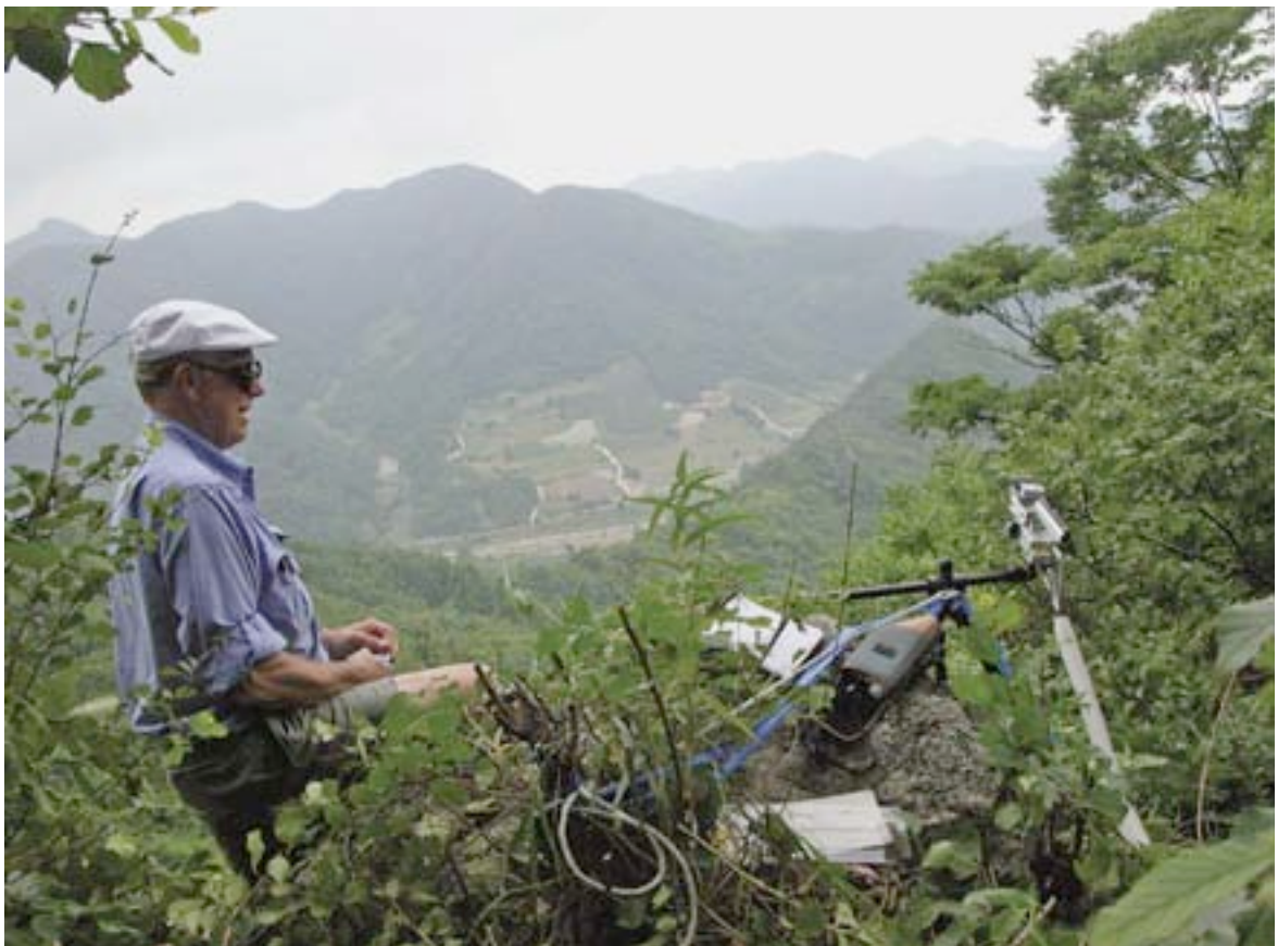
Tom Whitlow uses the LiCor 6400 to measure photosynthesis on a tree growing near the Buddhist hermitage at Podogam on Woraksan. The real-time photosynthetic rate (expressed as the rate of CO 2 ) is determined after inserting a leaf in the unit's cuvette, seen attached to a tripod on the righthand side of the image.
