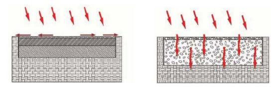
Figure 17. The left figure shows rain on a traditional asphalt parking lot- after it hits the surface it typically runs off into a storm sewer system. The right figure shows rain on a porous asphalt parking lot- after it its the surface it infiltrates through the pavement into the structural soil reservoir below. Water then infiltrates into the ground, recharging the groundwater over time. *Both figures by Ted Haffner.*
