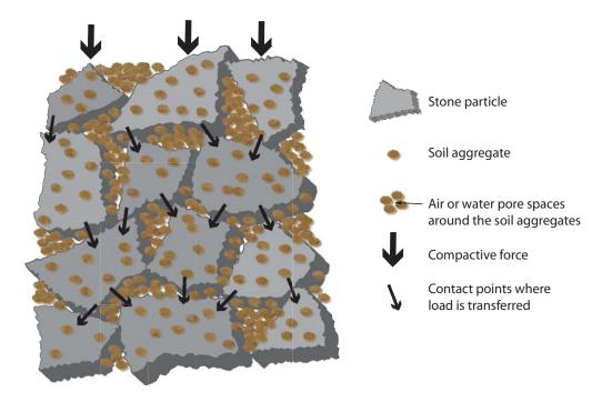
Figure 7. Conceptual diagram of structural soil including stone-on-stone compaction and soil in interstitial spaces.
