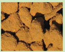
Figure 11. Davis Soil, a nonloadbearing soil (i.e. not a structural soil) with high infiltration rate and high potential for water storage. Photo by Qingfu Xiao.
