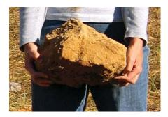
Figure 5. Compacted soil from a typical construction site. Lack of structure prohibits root penetration and growth. Photo by John W. Layman.
