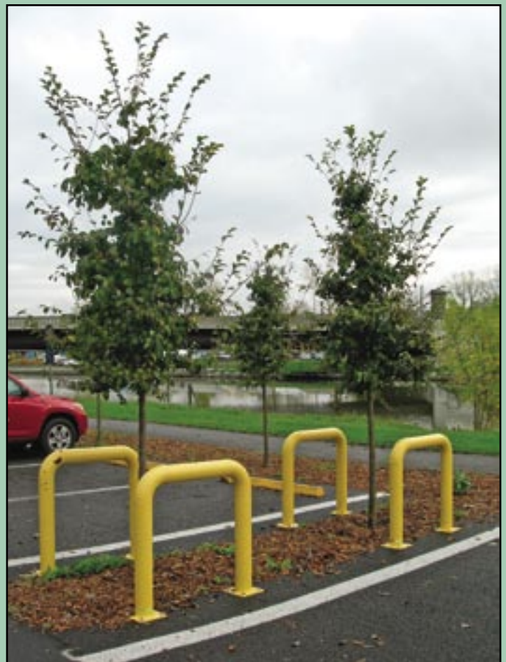
'Accolade' elms in the parking lot towards the end of their second year of growth in CU-Structural Soil overlaid with porous or traditional asphalt. All trees are doing very well, putting out one-and-a-half to two feet of new growth in their second year, with no differences due to surface treatment at this date. Evaluations will be ongoing.
