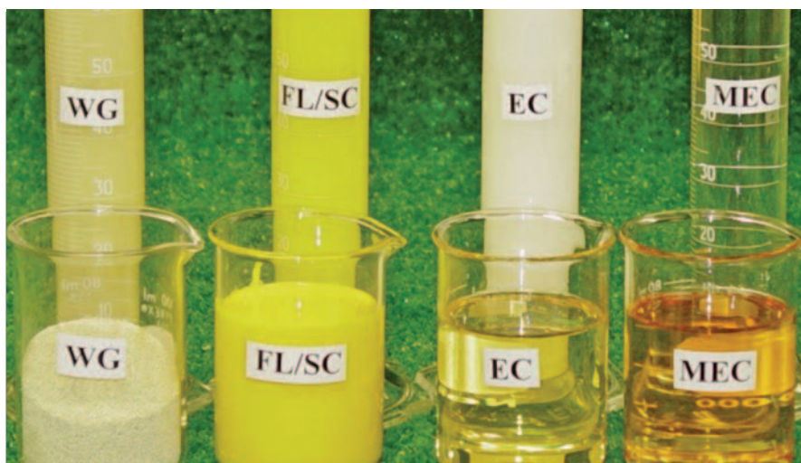
Figure 1. Formulations of pesticides used on turfgrass include (left to right): water-dispersible granule (WG), flowable or suspension concentrate (FL/SC), emulsifiable concentrate (EC) and microemulsifiable concentrate (MEC).
