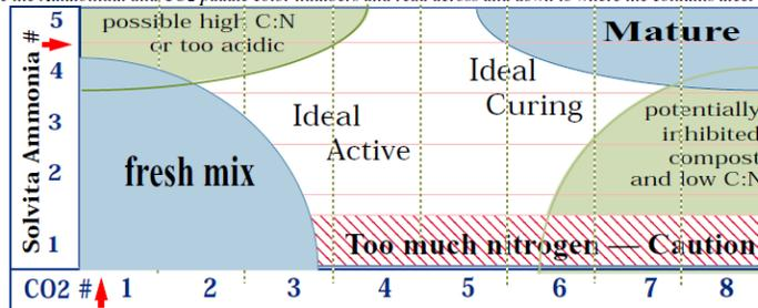
Example: If the NH<sub>3</sub> result is 2, and the CO<sub>2</sub> result is 6, then the process is Active moving into Curing
