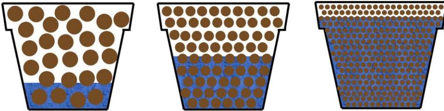
Water table height is only affected by particle size, not by container height
