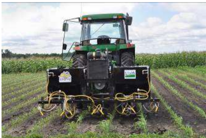
Tractor-mounted system for spraying corn grit to shred the leaves of weeds growing between crop rows. (D3204-1)
