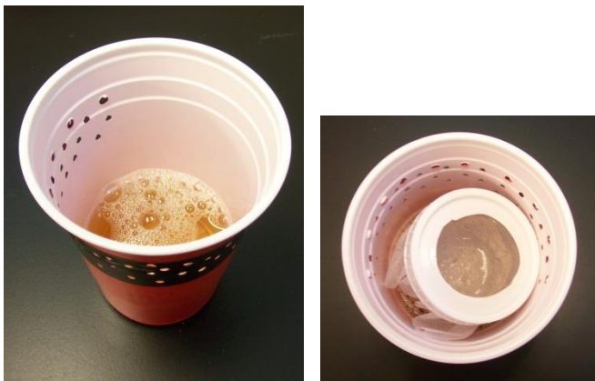
Viewed from above, the ampule fits inside cup and floats on the drowning solution.
