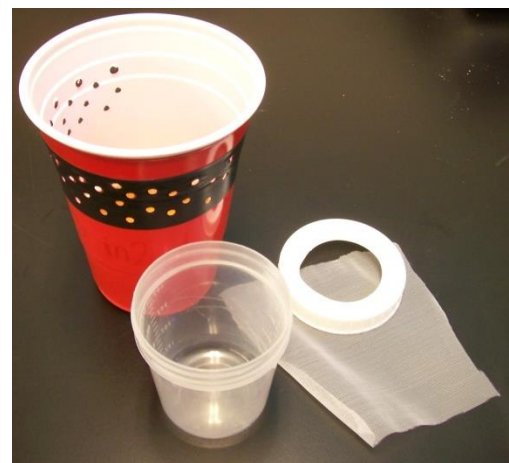
Red cup trap and specimen container assembly for the dough bait ampule.
