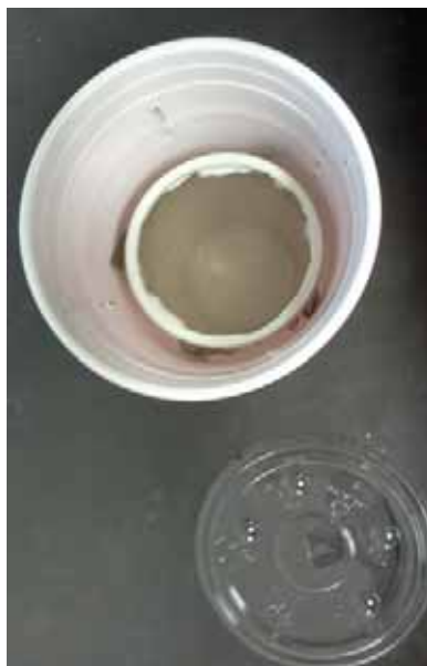
Trap components: specimen cup fits inside cup
