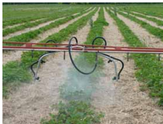
Close up of boom design with all 5 nozzles.
