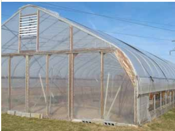
Fig. 1. Cool air from outside goes in the roll-up sides (right) and warm air in the highest parts of the tunnel flows out the gable vents.
