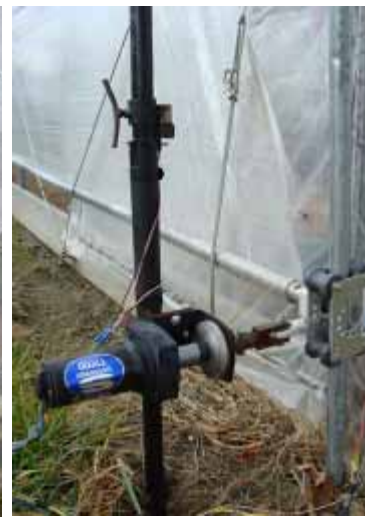
Fig. 3. Battery-driven motor that rolls up the tunnel sides below (left), and solar cell that maintains charge in the battery (below right).
