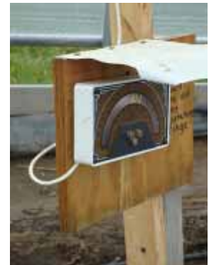
Fig. 2. Adjustable thermostat that controls roll-up sides of a high tunnel. Developed by Howard Hoover, high tunnel manufacturer, Penn Yan, N.Y.
