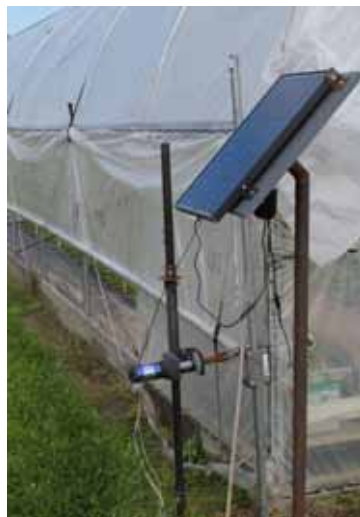
Fig. 3. Battery-driven motor that rolls up the tunnel sides below (left), and solar cell that maintains charge in the battery (below right).
