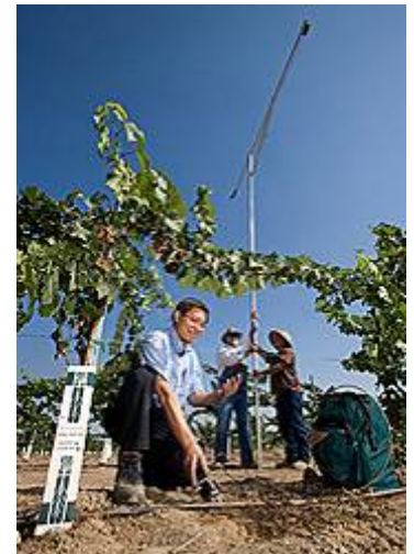
Soil scientist Dong Wang (left) records soil moisture data with a probe as technician Matt Gonzales (right) and agricultural engineer Jim Gartung record grape canopy cover with a spectral camera. Manually collecting data on the ground is necessary for calibrating satellite imagery.
