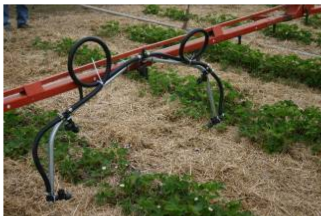
Cambridge NY Farmer John Hands' Boom Sprayer fitted with Dr. Andrew Landers' 5-nozzle hoop spray apparatus.
