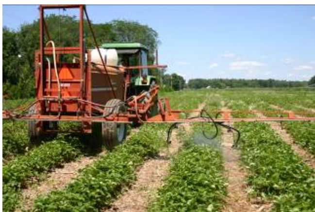
Cambridge NY Farmer John Hands' Boom Sprayer fitted with Dr. Andrew Landers' 5-nozzle hoop spray apparatus.
