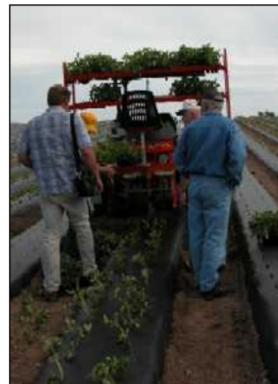
Figure 3: Planter for strawberry plant plugs.
