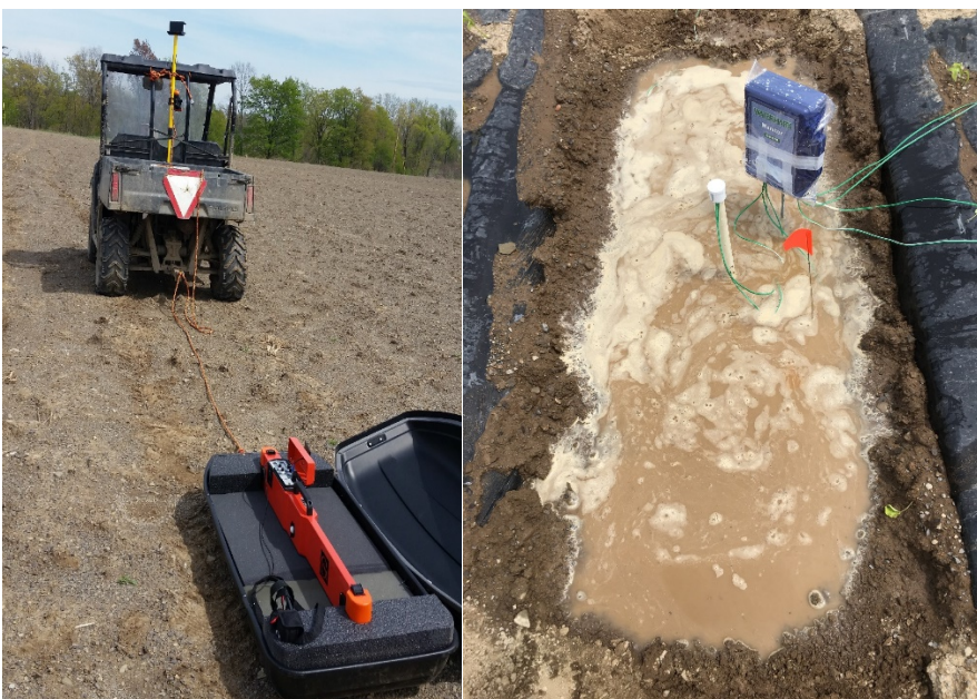
Figure 1: The electromagnetic instrument mounted in a sled that is drawn across the field for soil variability mapping and irrigation experiment with soil moisture monitoring at the 10 cm and 30 cm depth of the soil profile.
