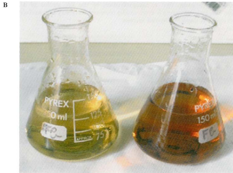
HARMAN ET AL. , FIG. 4. Degradation of polyphenolics from olive oil wastewaters by the activities of Trichoderma spp. The fungi were added to diluted (1:3 waste:water dilution) wastewater, the fungi were added and the content of polyphenolics in the mixture was followed over time. Phenolic compound content was determined by using the method of Folin-Denis based on the commercial substrate (Folin-Ciocalteu reagent; Sigma Scientific). A 5 ml total reaction mixture consisted of 250 \mu l of the reagent, 500 \mu l of sodium carbonate 20%, 100 \mu l of the sample to be tested, and distilled water. The phenolic concentration was determined based on a standard curve with differing concentrations of tannic acid. (A) The percentage degradation of the polyphenols; (B) the change in water color by the process. Analysis of variance of arcsine transformed percent values of all Trichoderma treatments were significantly different ( P < 0.05 ) from controls without the strains.
