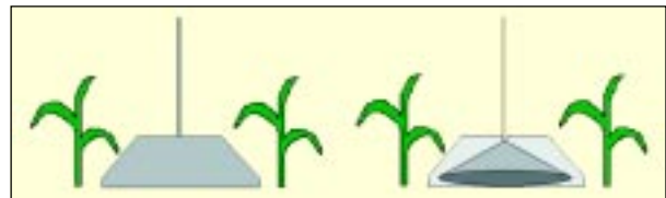
Figure 23. Shielded sprayer and spray pattern inside shield.
