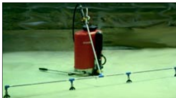
Figure 7. Four nozzle boom attached to a knapsack sprayer.
